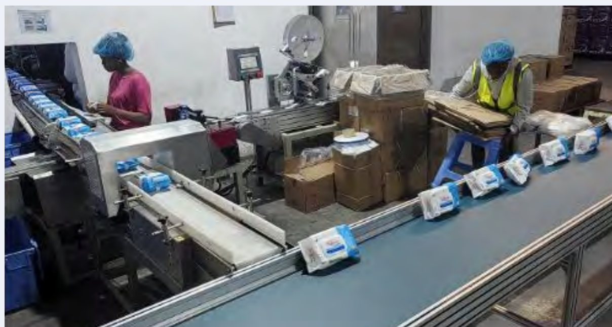
Automatic Identification and Rejection System for Wet Wipe Splices 濕巾接頭自動識別及剔除系統
